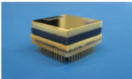
**Figure 4.** Detector with 20x20x10mm CZT crystal showing planar cathode and guard ring. (Courtesy of Quik-Pak, a division of Delphon Industries)
