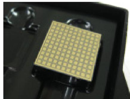
**Figure 6.** A crystal that was re-shaped and polished from an original highly irregular shape and then metallized with a solderable pixel pattern in a steering grid / guard ring arrangement. (Courtesy of Quik-Pak, a division of Delphon Industries)
