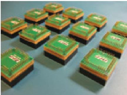
**Figure 1.** Completed detectors prepared for a large-scale array to be used in a space telescope application (Courtesy of Quik-Pak, a division of Delphon Industries)
