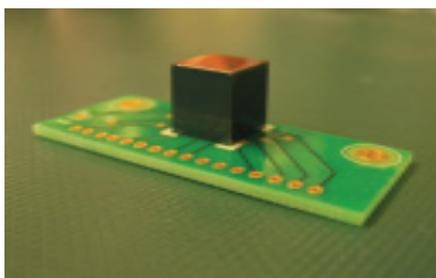
**Figure 2.** A detector assembly with 15mm crystal directly mounted for use in a high-energy experiment (Courtesy of Quik-Pak, a division of Delphon Industries)
