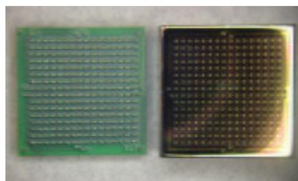
**Figure 5.** On the right is the high-density layout of anode pixels on the CZT crystal, surrounded by a guard ring and steering grid layout. On the left is the interposer with matching 300um bumps on a 500um pitch grid. (Courtesy of Quik-Pak, a division of Delphon Industries)
