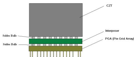
**Figure 3.** Representation showing the stack-up of the CZT, interposer and PGA connected with solder balls.
